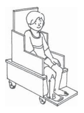
If you want to move the child around in the box seat, castors can be attached to the bottom of the seat so that it moves easily. If castors are attached, a foot rest will have to be added to the seat. To measure for the height of the foot rest, measure the child from the back of the ankle to the back of the knee (B to A).
