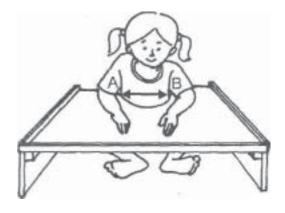
The cut-out portion should be measured to fit the child. The diameter of the semi-circle should be the width of the child's waist, plus two inches (A-B). It should fit comfortably around the child.
