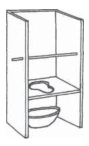
The height of the rod will be from the seat to just below the armpits. It should be at a distance of 2 inches in front of the child's chest.
